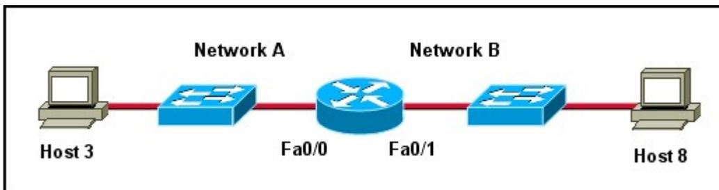
Refer to the exhibit. Host 3 on Network A is sending data to Host 8 on Network B. Which address is the default gateway of Host 3?
