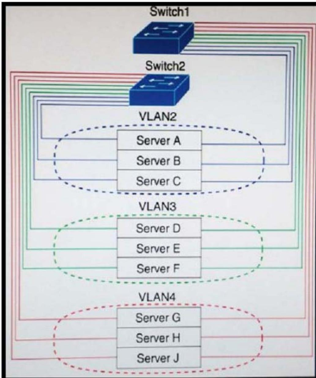
Two Layer 2 Cisco Nexus switches are connected to application servers in a data center. Server A cannot communicate with servers that are in VLANs 3 and 4, but it can communicate with server B and C.
